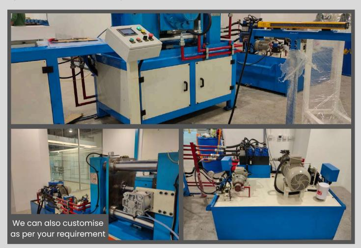
A Tube-expanding hydraulic Press with two cylinders is a specialized Machine designed for the R and D of the TATA Group. The purpose of this machine is to expand the ends of tubes from INSIDE; this is a special customized requirement.
