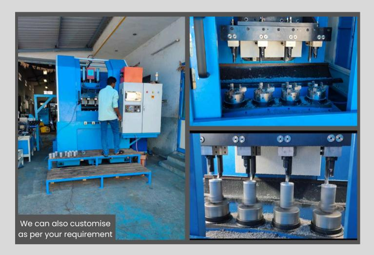
4 hydraulic chuck fixed in 4 spindle cnc lathe vertical lathe.
