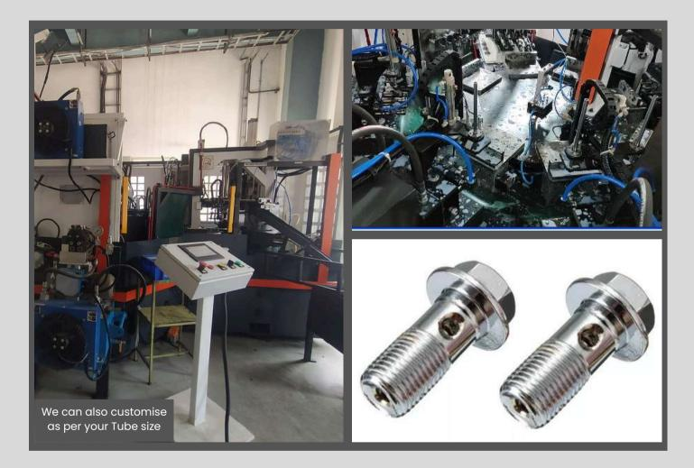
Banjo Bolt Turning and Drilling SPM, which has a cycle time of 4 to 5 seconds/part. With a single workforce, turning the Drilling machine automatic can operate both machines, improving productivity and increasing profits.
