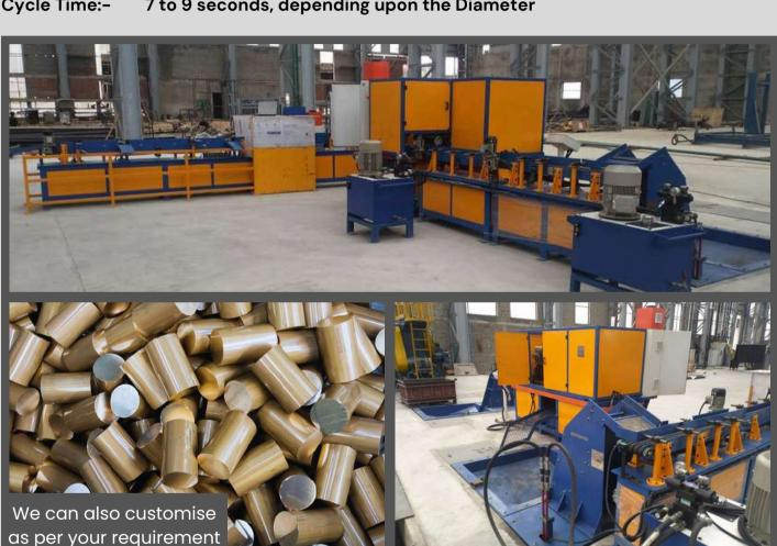
This machine does the Chamfering operation fully automatically. The billets will be put in the pit formed Step feeder system. From there, it moves to the machine for chamfering, automatically weighing inspection without manpower hindrance.
