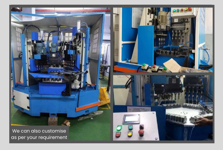
Drilling and Tapping machine, its designed and manufactured for high volume production, of Heat Sink and similar components. Many types of Aluminum Heat sinks, are widely used in industries, which normally requires Drilling and Tapping for fixing.
