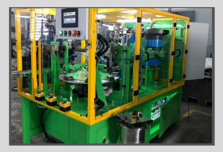
This is Heat sink assembly machine with I C. We need to put all part automatically including screwing it. Only I C has to be fed manually.
